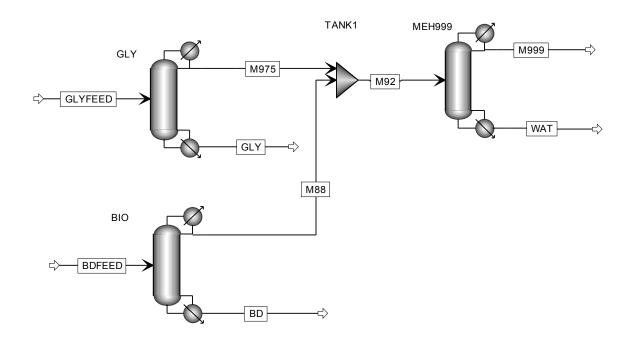
Sometimes separate evaporator is needed if water content in glycerin is greater 30% (by wt). BP grade Glycerin (99.5% wt) can be achieved by using vacuum batch distillation column.
